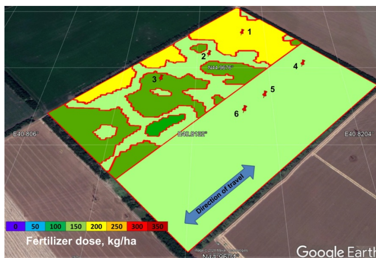
Figure 2. Task map for the first and second differentiated fertilizing of winter wheat with ammonium nitrate for field 11/1.
